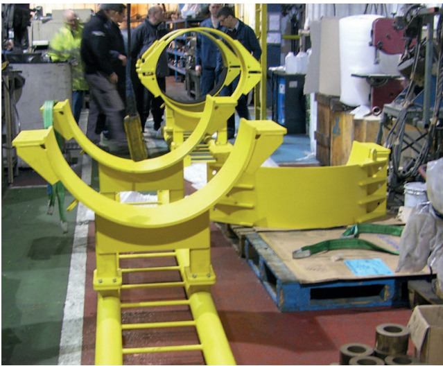
New ladder sections and clamps were fabricated, to be installed once blasting and coating work completed.
