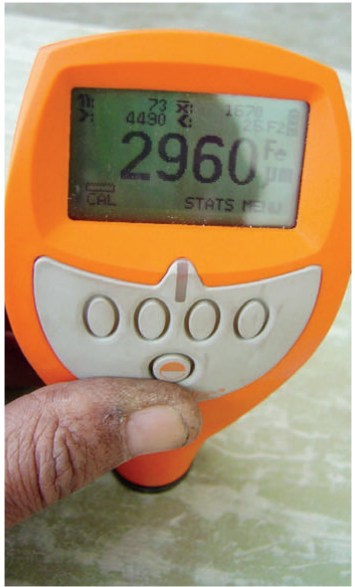
Paint thickness measurements, detailing readings with little or no wear of the solvent free resin. Taken 9 months later in the cargo.
