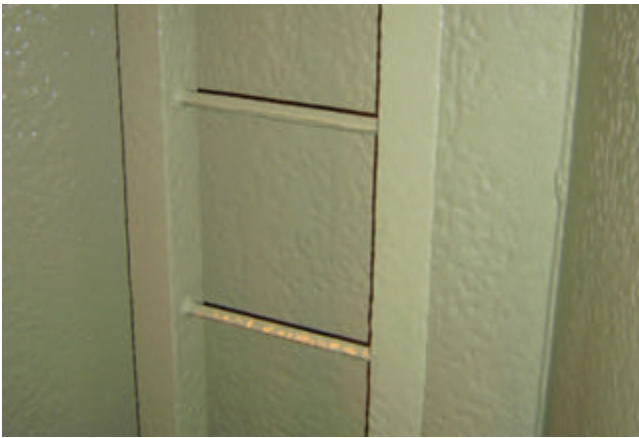
Fast set Urethane applied to cargo hold bulkheads and ladder sections to a thickness of 3mm (3,000 microns) in 1 single application.
