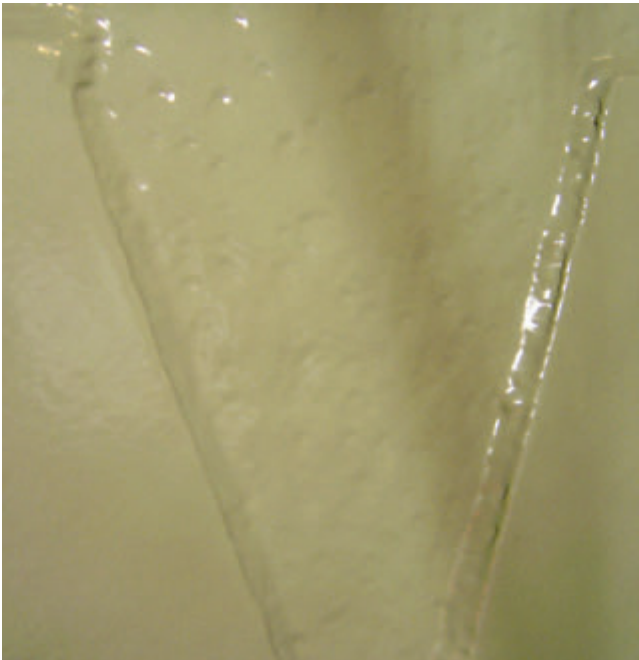
Fast set Urethane applied using plural component heated spray pump.
