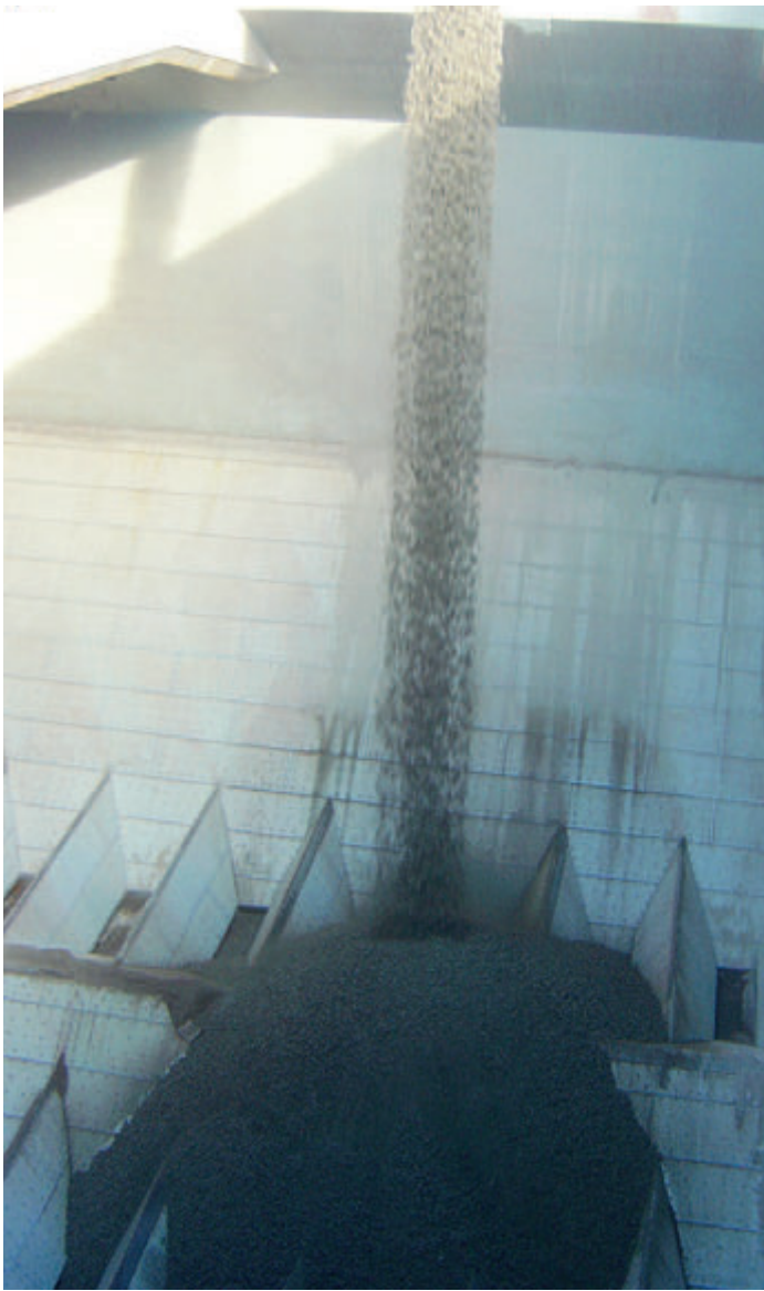
Granite loading into Urethane coated cargo holds.
