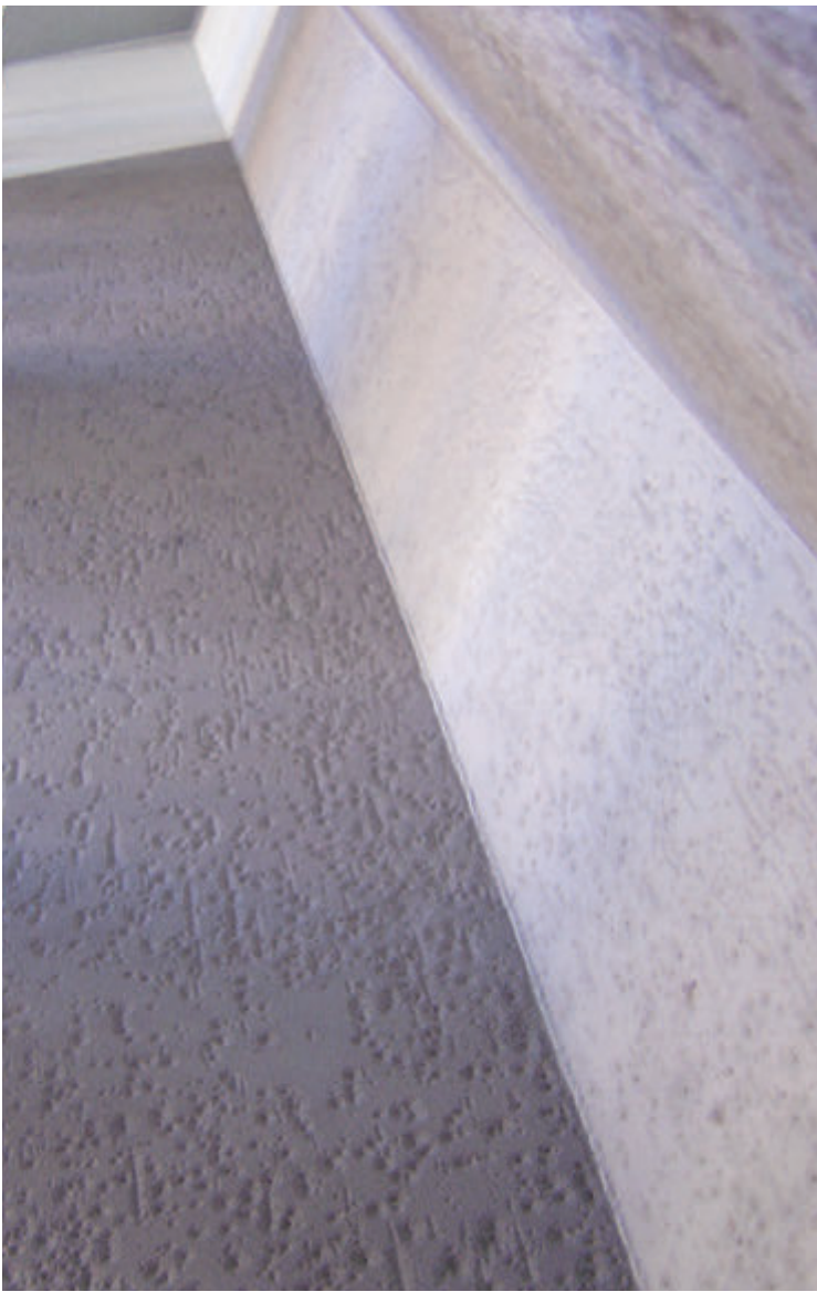
Corrugated bulkheads blasted to SA 2.5 standard prior to coating application.
