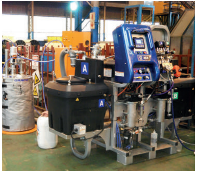
Fast set Urethane applied using plural component heated spray pump.
